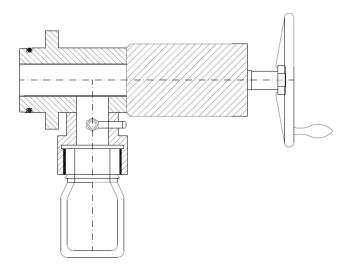
Purely suitable for liquid application where liquid flows freely in the Sampling Bottle by gravitational force. Very compact type of construction.
