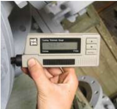
Paint Thickness Test
