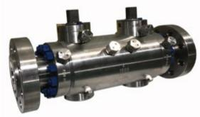
Machined from one piece or three piece "grain flow controlled" forging. This valve features two in-line ball pattern primary and secondary isolating valves with a heavy duty needle valve vent, offering "through to process" rodding in bore sizes from 15 mm to 600 mm (1/2" incto to 24"
