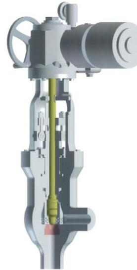
1. Easy and fast to change valve seats and cages damaged by erosion.
