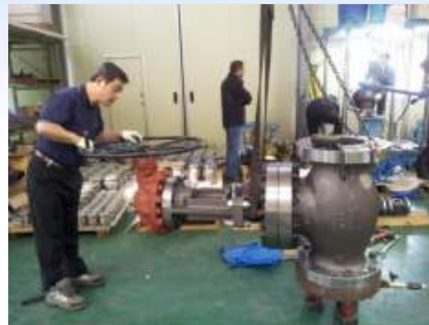
600LB GLOBE VALVE FUNCTIONING TEST
