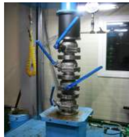
BALL VALVE HYDROSTATIC TEST
