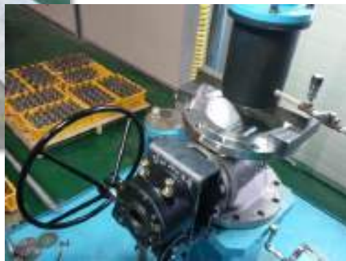
600LB GLOBE VALVE FUNCTIONING TEST
