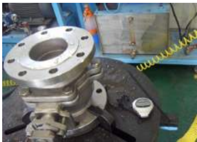
BALL VALVE PNEUMATIC SEAT TEST
