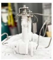
All Ladish cryogenic valves are tested in accordance to API 598. Our in-house test stands are capable of testing up to 24". Optional non-cold box and cold-box tests include:
