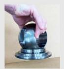
If uncoated metal balls and seats are in direct contact, they would be damaged due to galling when operated and would never seal well. It is the ball and seat coatings that provide the sealing and allow the
