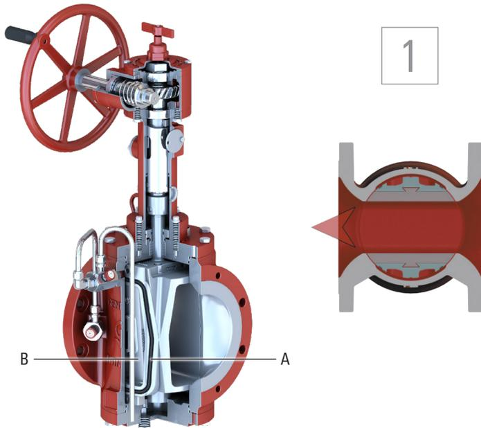
1. The seals (A) are permanently bonded into the slips (B), which are mounted on a central plug. In the open position, the slip seals are completely out of the flow.
