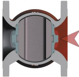
3. When the handwheel is turned farther clockwise, the tapered plug begins to lower, forcing the slips against the body and initiating the verifiable seal. Because its seals never drag in well-maintained valves, the GENERAL VALVE Twin Seal plug valve requires less torque to cycle.
