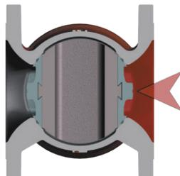
4. In the closed position, the slip seals are expanded, compressing the slip seals until metal-to-metal seating is effected. Because it is mechanical, the valve does not rely on line pressure differential to help make it seal and even seals in vacuum service.
