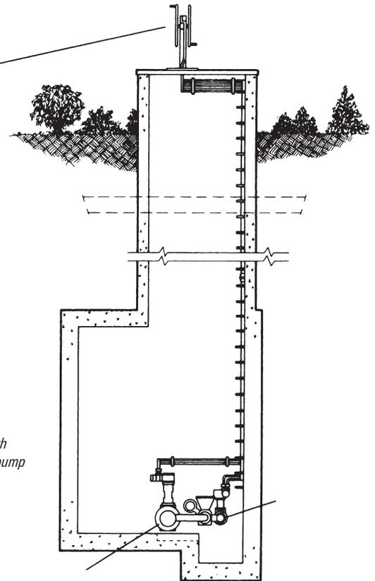
*Typical hydraulic extension systems are installed with two valves, featuring dual above-grade handwheel pump assemblies mounted on the same pedestal.*
