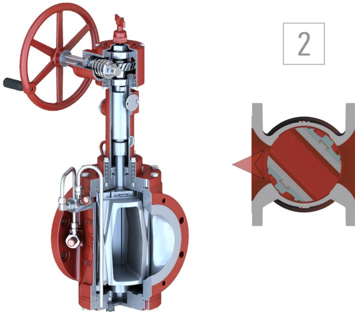
2. Turning the operator handwheel clockwise rotates the plug assembly 90° to block flow. During rotation, clearance is maintained between the seal and the valve body, enabling free movement and avoiding abrasion.
