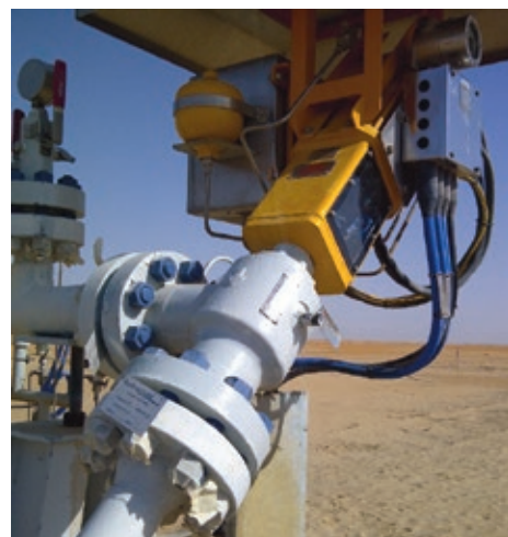
CC30 choke with linear hydraulic actuation
