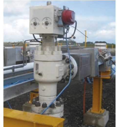
CC40 choke with hydraulic stepping actuation
