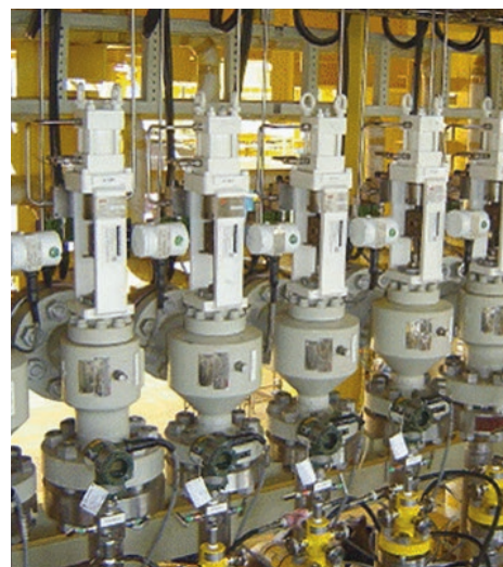
CC15 choke with linear hydraulic actuation
