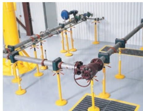
In addition to testing control chokes across a wide range of pressures, Cameron measures flow rates and noise in a flow loop per ISA specifications.
