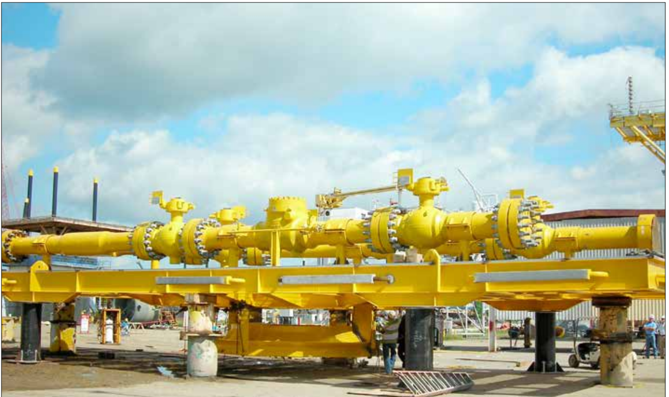
CAMERON ball valves and TOM WHEATLEY check valves are used for subsea production.
