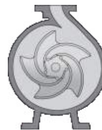
Expanding Volute Casing (Standard Pump)
