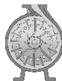
Circular Concentric Casing
