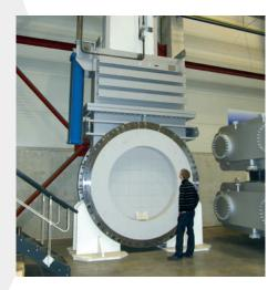
TRTs are specially designed low revolution turbines that use the hot gases from the blast furnace to generate power. The design has been optimised to reduce all drag and friction to produce a high efficiency turbine – 30 years' experience results in the lowest losses. They can simultaneously support two blast furnaces.
