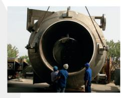
A key part of the process, our bottom unheading devices ensure reliable and (most importantly) remote safe unheading to optimise operational efficiency.
