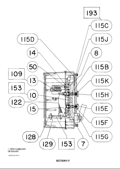
Figure 27. Gauge Block and Bypass Valve Assemblies
