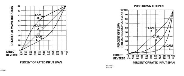
Figure 19. Flow Characteristics for the Various Cams When Used With an Equal Percentage Valve Characteristic Push-Down-to-Close Valve
