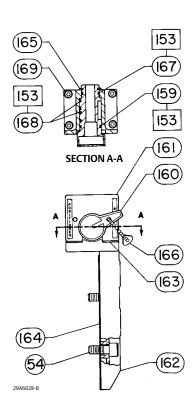
**BYPASS VALVE ASSEMBLY** FOR 3610J POSITIONERS
