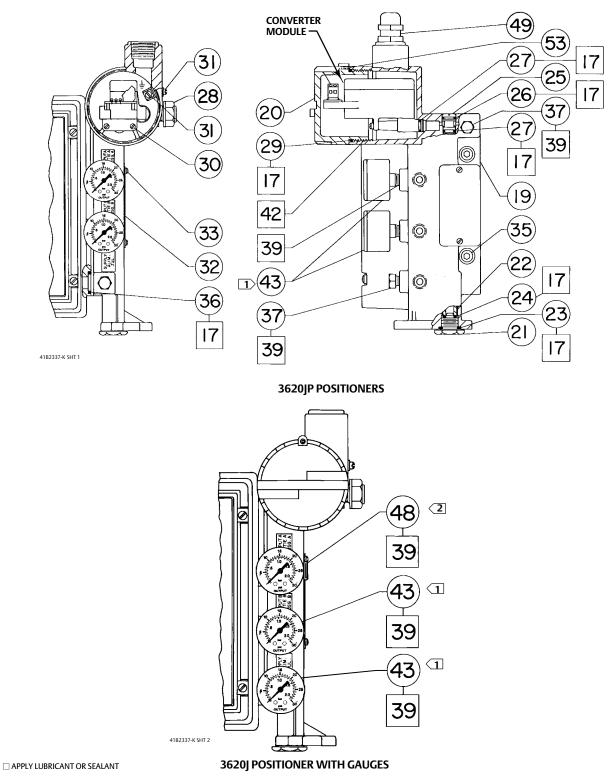
NOTE: D GAUGES MAY BE REPLACED BY PIPE PLUGS (KEY 37) OR TIRE VALVES (KEY 41) C KEY 48 IS USED FOR 3620J POSITIONER ONLY
