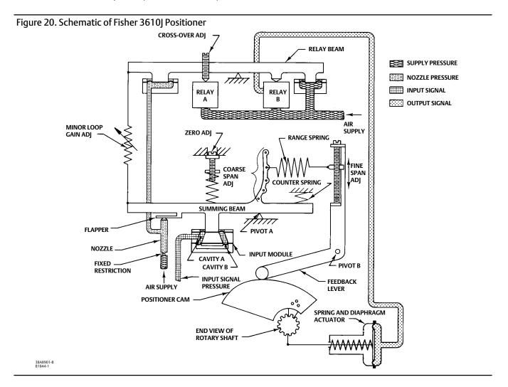
As a result, the actuator rod extends and the actuator rotary shaft rotates clockwise. This causes the feedback lever to pivot clockwise increasing the force applied to the summing beam by the range spring. This force, which opposes the downward force on the summing beam caused by the increasing input signal pressure, continues to increase until the summing beam torques are in equilibrium. At this point, the valve shaft is in the correct position for the specific input signal applied.
