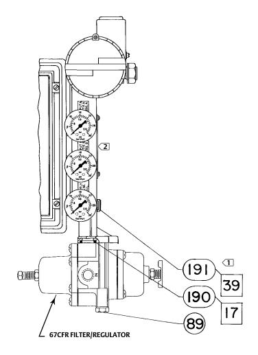
NOTES: THIS PIPE PLUG IS USED ONLY WITH INTEGRAL MOUNTED FILTER/REGULATOR. SEE FIGURE 31 FOR 3622 ELECTRO-PNEUMATIC CONVERTER KEY NUMBERS. 41B2337-K SHT 1
