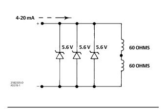
Figure 12. Fisher 3622 Converter Equivalent Circuit
