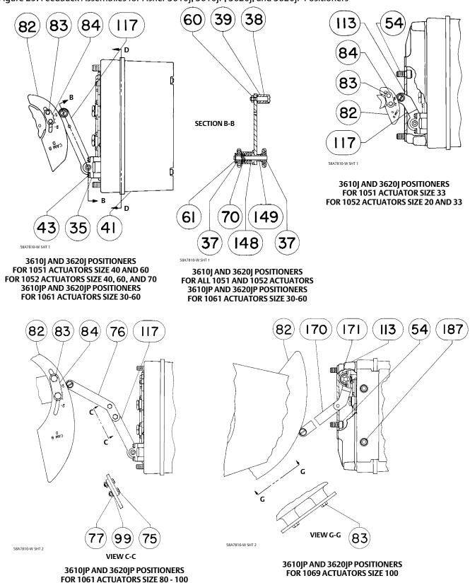
Figure 29. Feedback Assemblies for Fisher 3610J, 3610JP, 3620J, and 3620JP Positioners
