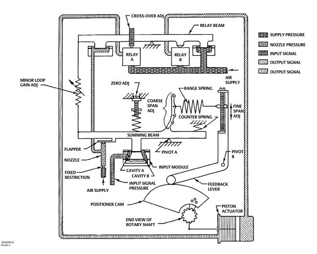
Figure 21. Schematic of Fisher 3610JP Positioner
