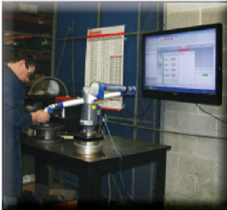
Coordinate Measuring Machine provide 3D data
