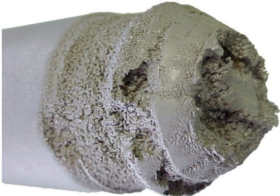
Control Valve Plug Damaged by Cavitation
