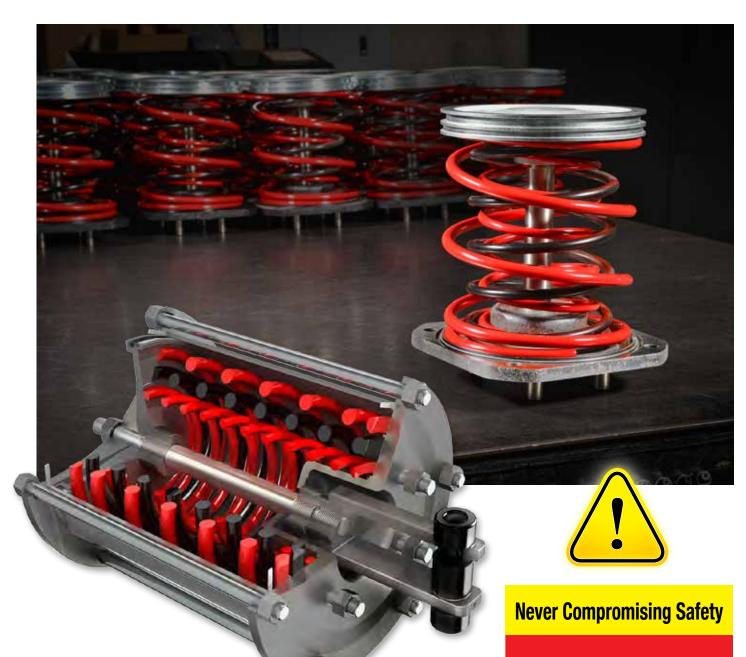
We feel strongly that our actuators shouldn't cause injury to anyone. Thus, we have made safety an integral part of our actuator design, specifically the springs, which can cause serious harm to personnel or damage other equipment if not captured. All QTRCO springs are captured and contained within the force module even if the end cap and cylinder are removed.
