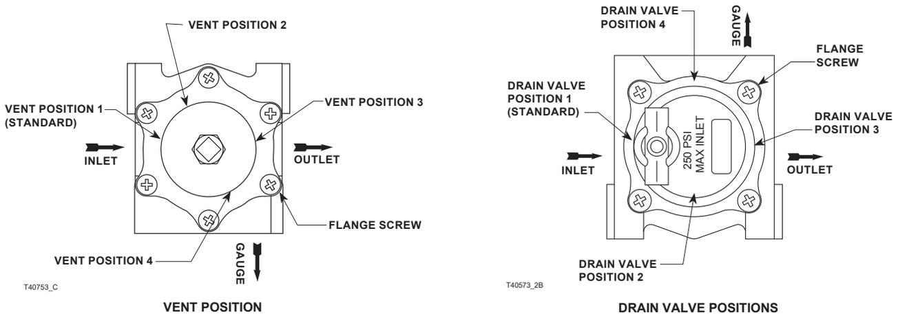
Figure 4. 67C Series Vent and Drain Valve Positions
