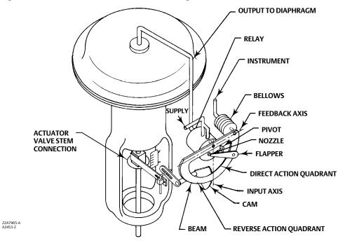
Figure 6. Fisher 3582i Positioner Schematic Diagram
