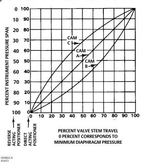
Figure 8. Equal Percentage Valve Flow Characteristics as Modified by Various Cams
