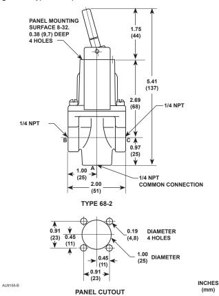
Figure 3. Type 68-2 Switching Valve Dimensions
