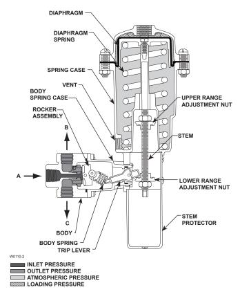
Figure 2. Type 168 Operational Schematic
