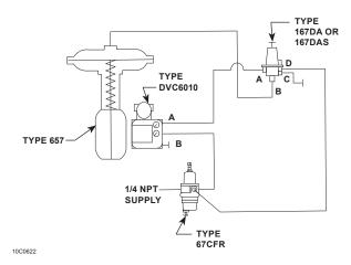
Figure 3. Typical 167DA or 167DAS Installation (Lockup system using Type 167DA or 167DAS to close air circuit to diaphragm of main valve in case of plant air failure. Main valve will remain in
