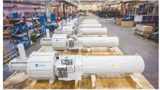
Quarter turn actuators for power & desalination project
