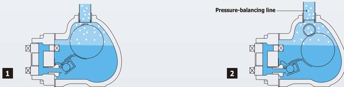
At start-up condensate enters the air trap. The float is rising and the condensate will be discharged through the wide open valve. Air, which usually enters the trap body together with the condensate, will accumulate in the upper part of the trap body. To prevent air locking, a pressure-balancing line connects the upper part of the trap with the drained equipment, so that the air can escape easily from the trap body.
