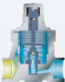
On start-up, the bimetal discs are all flat and the valve shaft is up with the valve fully open. Virtually all cold condensate and air are discharged.
