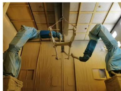
Kubota Construction Machinery (WUXI) Co., Ltd. (China) has increased quality and productivity while reducing revision of painting work by introducing painting robots. This has led to a reduction in the amount of paint used, and the amount of VOC emissions.
