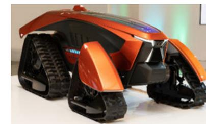
Concept model for a completely driverless BEV tractor announced in January 2020
