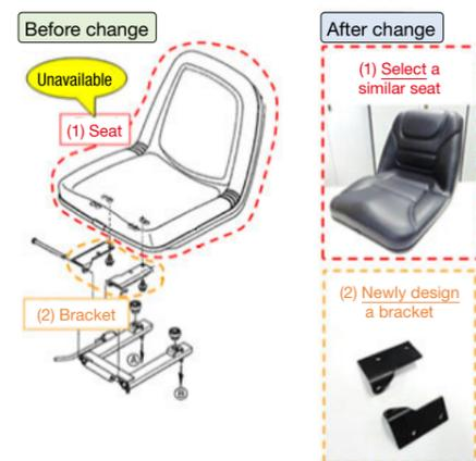
In addition to redesigning the part itself, we also conduct activities to enable substitution by selecting similar parts and designing new parts to ensure the part can be mounted compatibly.
