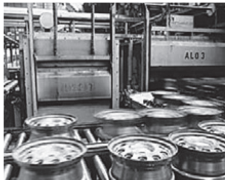
Aluminium industry: curing oven for wheel rims
