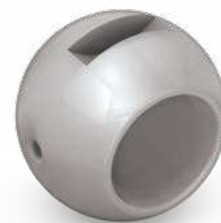
3 mm relief hole face the upstream
