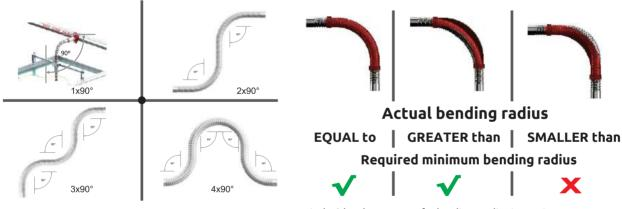
Use Fivalco<sup>®</sup> bend snap-gauge for bending gradius inspection
