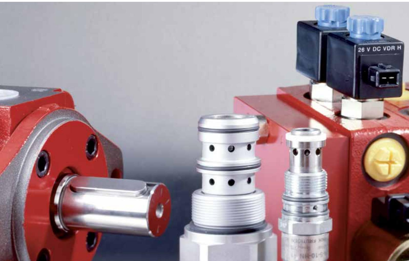
These lightweight aluminium valves are suitable for controlling single or double acting actuators. They are particularly suited to applications which demand a high degree of leak tightness. They are directly controlled 2/2 bi-directional seat valves which are solenoid operated. Their purpose is to control the feed and return pipes on hydraulic equipment with virtually zero leakage.
