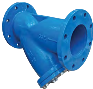
CI YST CAST IRON Y STRAINER FBE Coated S/S Screen Flanged AS2129 Table E 50mm to 600mm 100mm & 250mm available Table D
