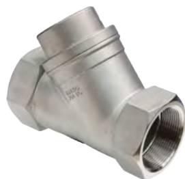
VPC PISTON CHECK VALVE 316 Stainless Steel Inclined PTFE seat 40 Bar Female BSP 8mm to 50mm
