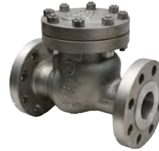
SSCK300 SWING CHECK VALVE 316 Stainless steel Stellite seat Flanges to ASME 300 15mm to 150mm
