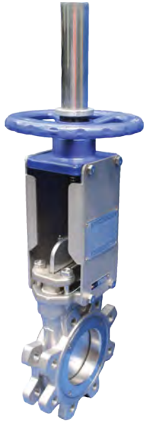
BKGV-E LUGGED TABLE E KNIFE GATE 316 Stainless Steel EPDM or METAL seat 1000Kpa 50mm to 600mm
