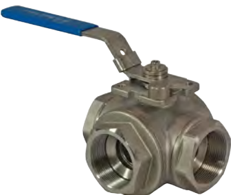
3WAYL/3WAYT 3 WAY BSP 316 Stainless Steel Reduced Bore L or T port Lockable lever PTFE seats 8mm to 80mm BSP 1000 PSI
