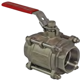
V3HT 3 PIECE BALL VALVE HIGH TEMPERATURE 316 Stainless Steel Full Bore Lockable lever operated High temperature seats 8mm to 100mm BSP 1000 PSI
