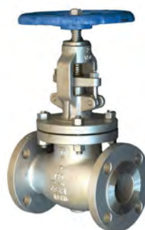
SSGL-150/300 FLANGED GLOBE VALVE ANSI 150 or ANSI 300 316 Body, STELLITE seat OS&Y Graphite Packing Spiral Wound Gasket 15mm to 300mm
