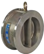
DUO 316-150 WAFER DUO CHECK VALVE 316 Stainless Steel Wafer to suit ANSI 150 Viton seats 40mm to 600mm Wafer Style
