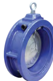
UNI CI CAST IRON WAFER CHECK NBR seat FBE Coated Body 304 SS Disc Suit AS2129 Tab E 50mm to 600mm
