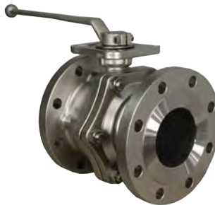
SS2020D-150 2 PIECE FLANGED ANSI 150 BALL VALVE Firesafe Certified ISO Direct Mount 316 Stainless Steel Full Bore TFM1600 seats 15mm to 300mm Lockable lever to 150mm Gear operator over 150mm
