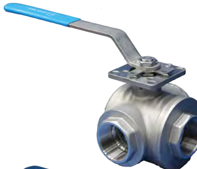
3WAYL/3WAYT -ISO 3 WAY BSP 316 Stainless Steel High Temp TFM1600 seat Full Bore L or T port ISO MOUNT Lever operated 8mm to 50mm BSP 1000 PSI
