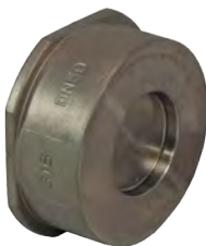
WVC 316 WAFER SPRING CHECK VALVE 316 Stainless Steel—Single Disc Suitable for a wide range of flange tables Rated to 40 bar 15mm to 100mm Wafer Style
