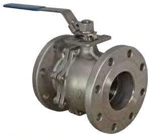
V2F-150 2 PIECE FLANGED ANSI 150 BALL VALVE 316 Stainless Steel Full bore 15mm to 300mm Also available drilled AS2129 Table E And undrilled
