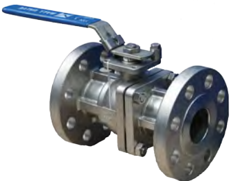
SS2020N-300 2 PIECE FLANGED ANSI 300 BALL VALVE Firesafe Certified 316 Stainless Steel Full Bore TFM1600 seats 15mm to 250mm Lockable lever to 150mm Gear operator over 150mm
