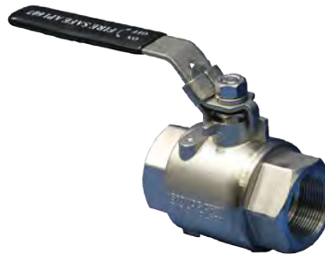
2006 Series 2 PIECE BALL VALVE Firesafe Certified Lockable lever operated 316 Stainless Steel Full Bore, PTFE seats 2000 PSI 8mm-25mm NPT 1500psi 32 to 50mm NPT 1000psi 80 to 100mm NPT
