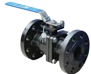
V3FSFB/RB 3 PIECE BALL VALVE Firesafe Certified, ISO PAD Lockable lever operated 316 Stainless Steel Full bore / Reduced bore PTFE seats 8mm to 50mm NPT 2000 PSI
