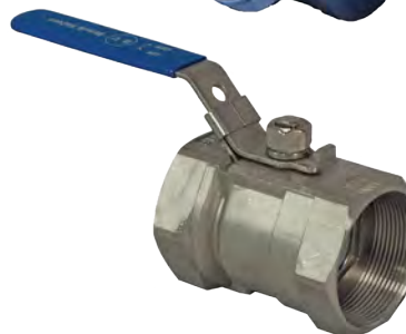
V1 1 PIECE BALL VALVE 316 Stainless Steel Reduced Bore Lockable lever PTFE seats 8mm to 50mm BSP Also available with NPT thread 1000 PSI
