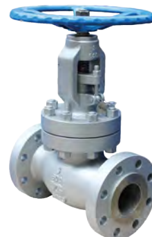
SSGL-150/300 FLANGED GLOBE VALVE ANSI 150 or ANSI 300 316 Body, STELLITE seat OS&Y Graphite Packing Spiral Wound Gasket 15mm to 300mm
