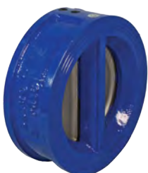
DUO CI CAST IRON WAFER CHECK VALVE EPDM seat FBE Coated Body 316 SS Plates Suits AS2129 Table E 50mm to 750mm
