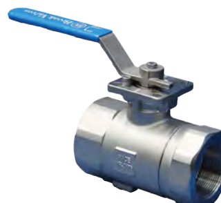
V2-3000 2 PIECE BALL VALVE 316 Stainless Steel Full Bore ISO MOUNT 3000 PSI Lockable lever Delrin seats 8mm to 50mm NPT
