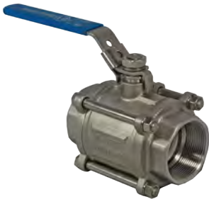
V3 3 PIECE BALL VALVE 316 Stainless Steel Full Bore Lockable lever operated PTFE seats 8mm to 100mm BSP 1000 PSI ... Available in NPT
