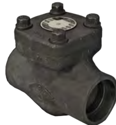
CP800 PISTON CHECK VALVE API 602 A105N Stellite seats CLASS 800 (2000psi) NPT or socket weld 15mm to 50mm
