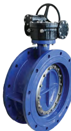
FSD CS (also Stainless non firesafe) HIGH PERFORMANCE BUTTERFLY VALVE PTFE seat ASME B16.5 150 and 300 LB Firesafe Certified, Manual or Actuated -40 to 250 Deg C 80mm to 600mm 150lb 80mm to 450mm 300lb
