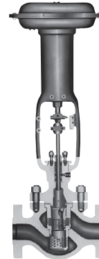
High pressure service low-noise cage type double seated control valve
