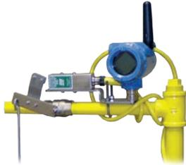
The TopWorx™ Wireless Safety Shower Monitoring Solution combines two 10 Series, latching GO Switches with a Rosemount 702 Wireless Transmitter that provide on/off indication, time stamping, and automated reporting functions for safety shower/eyewash stations.
