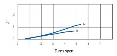
A =  $\frac{1}{4}$  inch (6.4 mm) orifice, valve C<sub>V</sub> 1.4 maximum B =  $\frac{3}{16}$  inch (4.8 mm) orifice, valve C<sub>V</sub> .83 maximum
