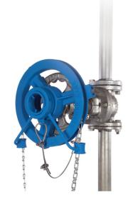
Maintain Handwheel and Operator - Retention of the chain wheel operator on valve stem is dependent on the handwheel remaining on the valve stem. The handwheel retaining nut MUST be secured with a set screw.
