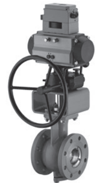
Type 82.7 Rotary Plug Valve with Type AT Rotary Actuator and Type 3730 Positioner
