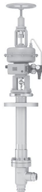
Type 3248-1 Cryogenic Valve, aluminum angle valve with positioner, supply pressure regulator, pressure gauges and additional handwheel
