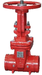
Resilient Seated OS&Y Type-Groove-Groove Ends Fig.333GG Standard:AWWA C515/BS5163 Size:DN50~DN300
