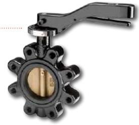
Crane Fluid System butterfly valves are compact quarter turn valves. The body is elastomer lined providing a resilient bubble tight shut off. The valves are supplied in wafer or lugged variants and may be lever or gearbox operated. Linings are EPDM or Nitrile rubber depending on the intended service conditions. Primarily recommended for on off service, they may also be used for non-critical throttling applications. Only a quarter turn is needed to fully open or close the valve.
