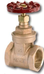
Crane Fluid System gate valves offer the ultimate in dependable service wherever minimum pressure drop is important. They serve as efficient isolation valves with fluid flow in either direction. The straight through design offers little resistance to flow and reduces pressure drop to a minimum. A gate-like disc - actuated by a stem screw and handwheel - moves up and down at right
