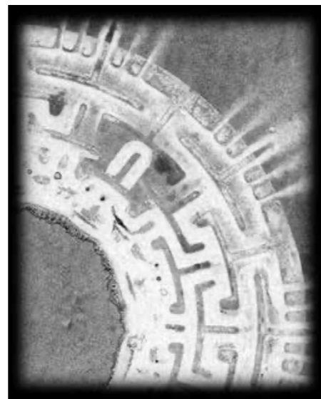
TEST CASE SHOWING SEVERE BLOCKAGE. ALL INLETS AND OUTLETS STILL IN USE. NEGLECTIBLE LOSS IN CV.
