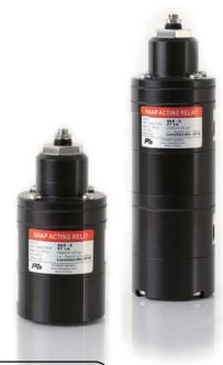
Snap Acting Relay is the device which is usually used with an air tank, converts an air flow direction and moves the valve to the fail-safe position when the signal air pressure is lower than the set air pressure. Also, it has a fail-freeze function to help the valve stay at the last position on the loss of a supply air pressure.
