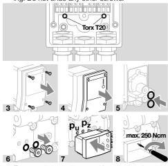
→ For more information on wiring, testing the tightness and commissioning, see enclosed "Tightness control TC 1, TC 2, TC 3" operating instructions. **9** After completing the wiring, tightness test and commissioning for the TC, refit the housing cover on the TC.
