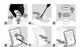
→ Remove the M20 cable gland or other type of connection.
