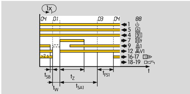
If the BCU detects a flame failure after a minimum operating time of 2 s, the valves are closed and the operation signalling contact is opened within time  $t_{SB}$ .
