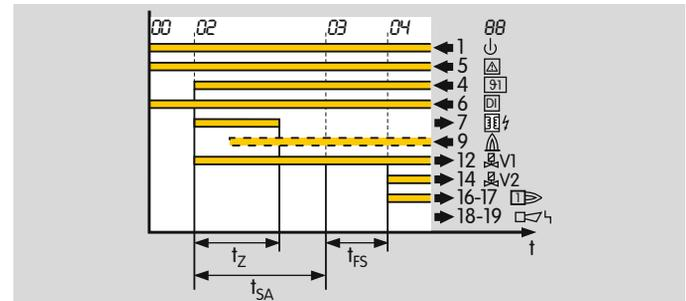
If the temperature in the furnace chamber drops below 750°C, the DI input must be disconnected from the electrical power supply and the furnace must be operated with the internal flame control system.
