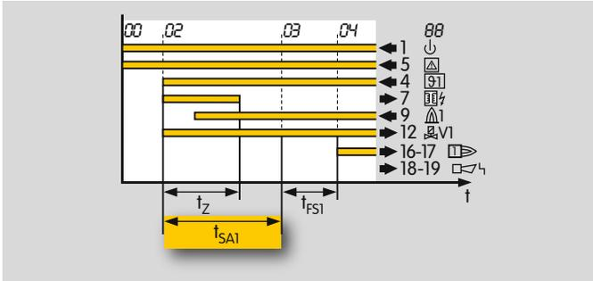
This indicates the safety time on start-up  $t_{SA1}$  for the pilot burner.
