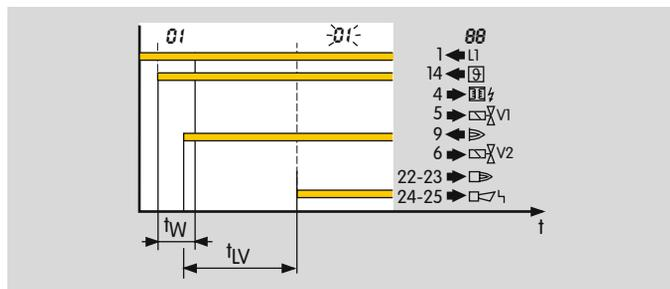
An extraneous signal (flame simulation) is a flame signal that is detected, although there should be no flame according to the program sequence. If such an extraneous signal is detected, the flame simulation delay time  $t_{LV}$  starts to elapse. If the flame simulation is discontinued during the flame simulation delay time  $t_{LV}$ , start-up can be initiated or operation continued. Otherwise, a fault lock-out occurs.
