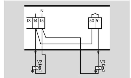
The opposite application describes a two-stage-controlled burner without a pneumatic air/gas ratio control system. The third gas valve (V3) and the air valve are activated simultaneously. During purging/cooling, the gas valve (V3) is not activated.
