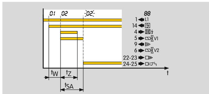
Once the start-up signal  $\vartheta$  has been applied, the waiting time  $t_W$  starts to elapse. During this time, a self-test is conducted to detect errors in internal and external circuit components. If no malfunction is detected, the burner will start up.
