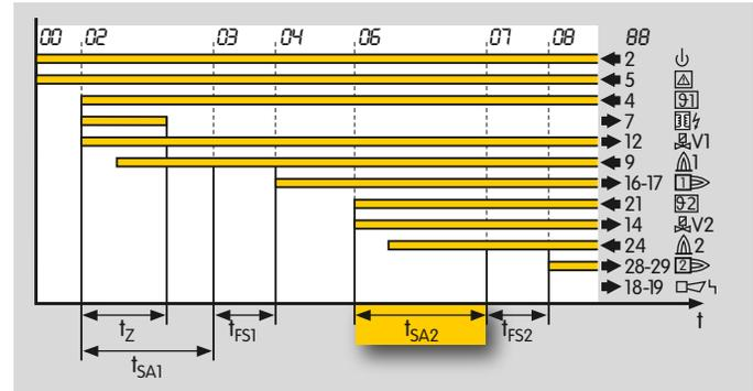
This indicates the safety time on start-up  $t_{SA2}$  for the main burner.
