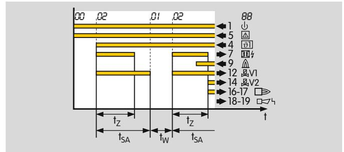
If several start-up attempts are set at the works and if the BCU detects a flame failure during start-up, it closes valve V1 after the safety time  $t_{SA1}$  has expired and attempts to start up again. After the last programmed start-up attempt has been completed, the burner control unit conducts a fault lock-out. The display blinks and shows the cause of the fault.
