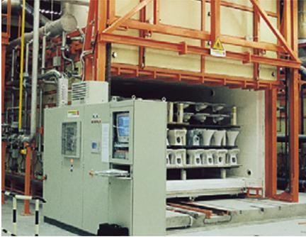
*Walking beam furnace with overhead firing*
