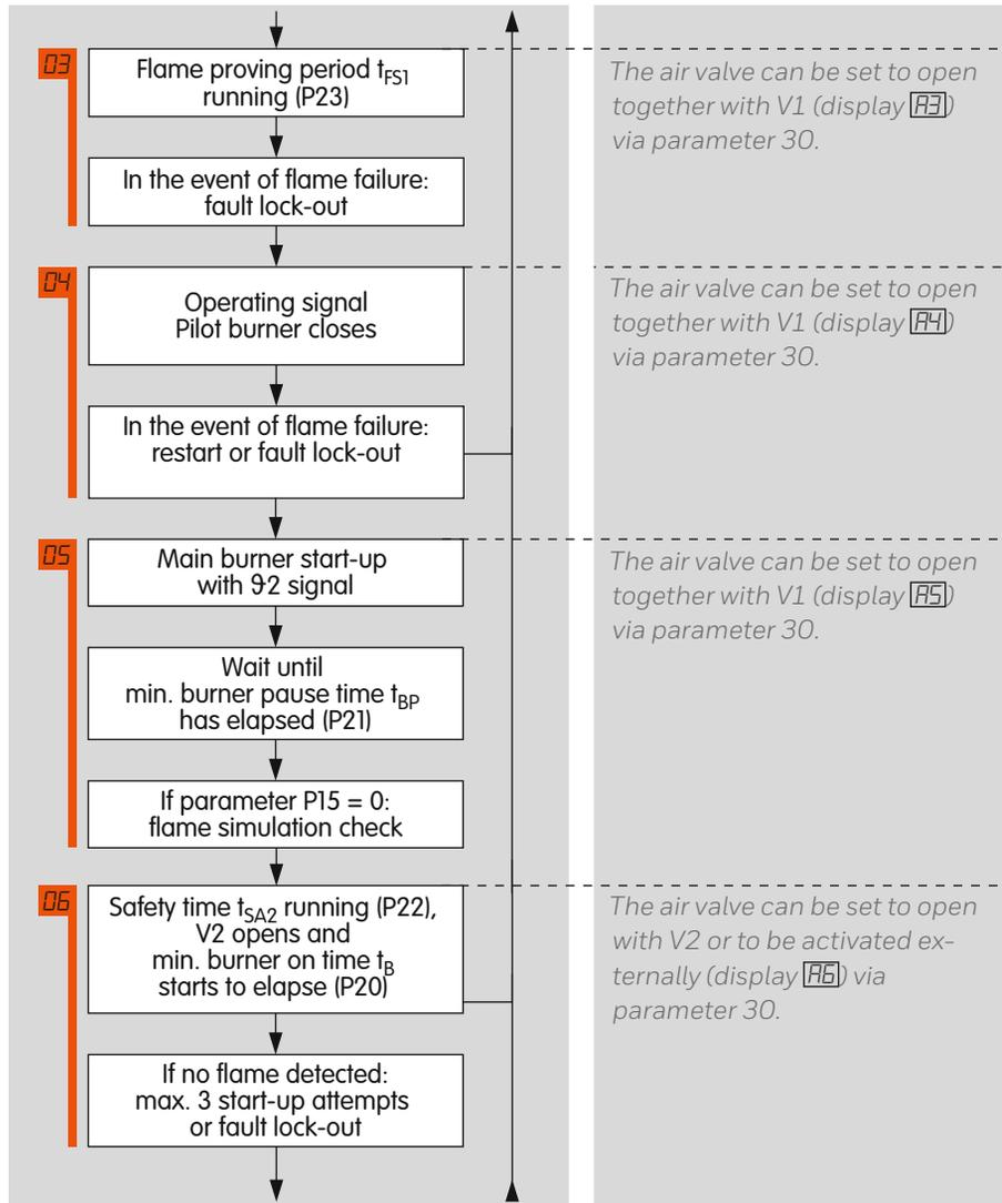
The BCU coordinates the correct program run for the pilot and main burners. The main burner can be started via the signal input “Start-up signal  $\vartheta 2$ ” (terminal 21) if required.
