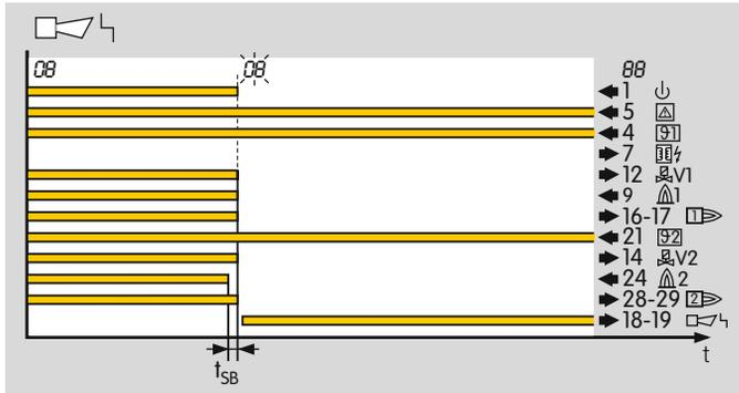
If the flame fails during operation, the valve outputs are disconnected within the safety time  $t_{SB}$ .
