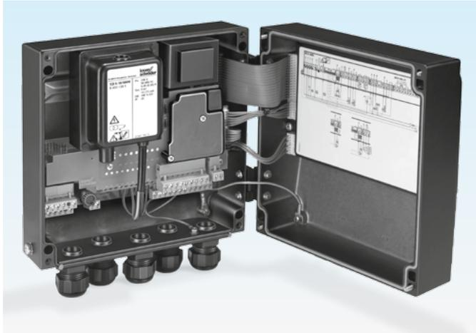
*The BCU unites the functionally interrelated components of automatic burner control unit, ignition transformer, Manual/Automatic mode and display of operating and fault statuses in a compact metal housing.*
