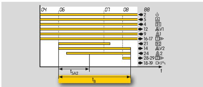
In the case of pilot/main burner monitoring, the minimum burner on time only has an effect on the behaviour of the main burner. The minimum burner on time for the pilot burner is limited to the safety time on start-up ( $t_{SA}$ ).
