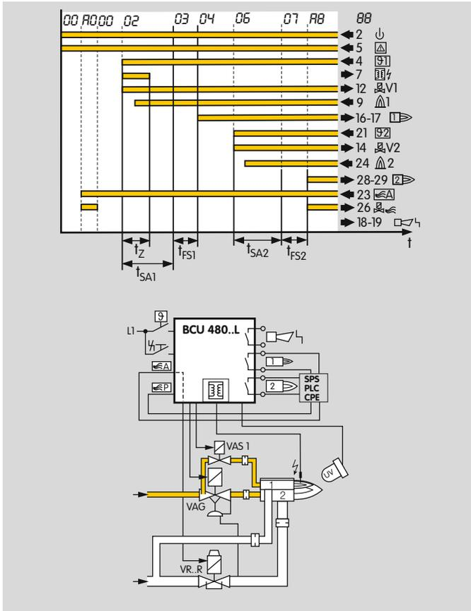
Parameter 30 = 0: The air valve opens if it is activated externally via input 23.
