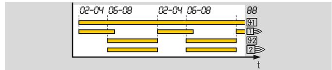
The pilot burner is switched off during the main burner safety time  $t_{SA2}$ . This type of flame control is required if no distinction can be made between the flame signals of the pilot and main burners (e.g. if both burners can be monitored with a single UV sensor). If the start-up signal for the pilot burner is applied continually, the pilot burner restarts immediately after the main burner has been switched off.
