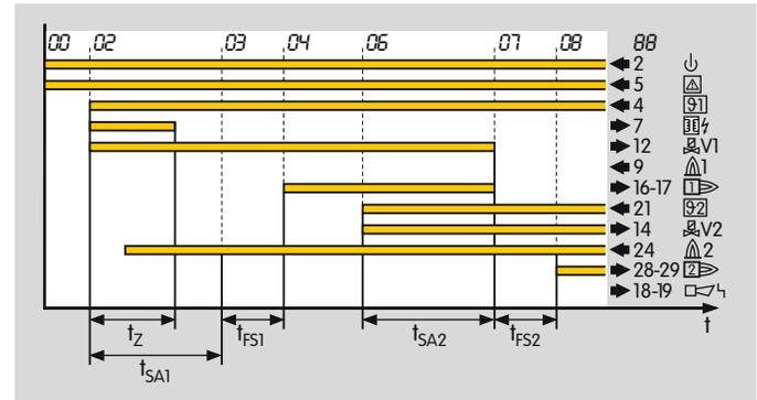
Operating mode: Interrupted pilot burner
