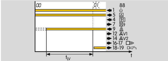
If the BCU notices an extraneous signal during the flame simulation check, it starts the flame simulation delay time  $t_{LV}$  (25 s). If the extraneous signal is discontinued during this period, the burner can start up. Otherwise, a fault lock-out occurs. [1] blinks on the display if an extraneous signal is detected by the pilot burner and [5] blinks if an extraneous signal is detected by the main burner.
