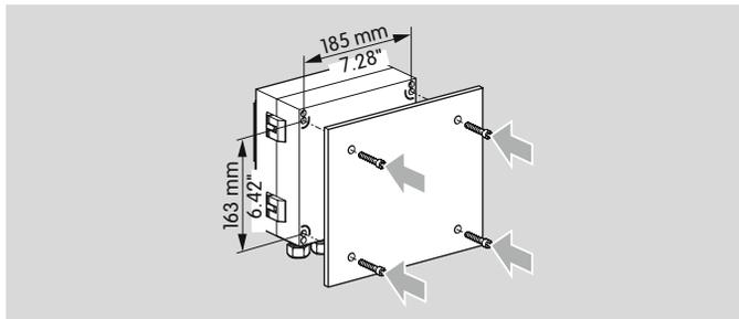
Screw on the closed unit to the rear with 4 self-tapping screws (enclosed).
