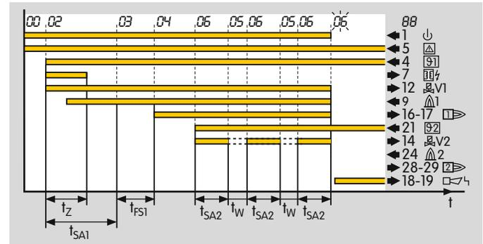
If several start-up attempts are set at the works and if the BCU does not detect a flame signal during start-up, it closes valve V2 after the safety time  $t_{SA2}$  has expired and attempts to start up again. After the last programmed start-up attempt has been completed, the burner control unit conducts a fault lock-out. The display blinks and shows the cause of the fault.
