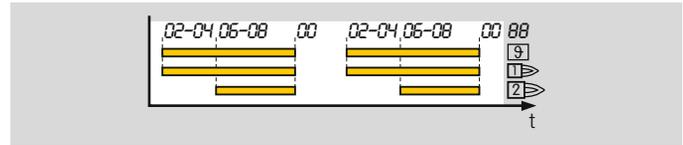
Pilot and main burners are controlled with one start-up signal (terminals 4 and 21 in parallel). The main burner starts automatically after the operating signal from the pilot burner has been detected. Operation is terminated simultaneously for both burners.
