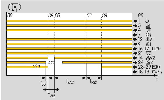
If the BCU detects a flame failure after a minimum operating time of 2 s, valve V2 is closed and the operation signalling contact is opened within time  $t_{SB}$ .
