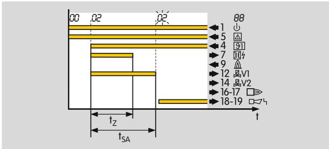
If no flame forms during start-up, a fault lock-out is performed after expiry of time  $t_{SA}$ . The display blinks and shows the cause of the fault.
