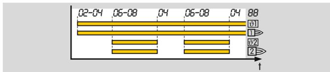
For applications which require a high system availability or where a continuously burning flame is necessary. The pilot burner is ignited once and remains constantly in operation. The main burner is controlled separately.
