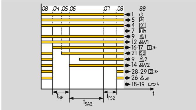
An immediate restart of the burner after a controlled shut-down, a start-up attempt, restart, cooling or purging is prevented by the pause time. The pause time starts when the air valve is switched off. If a start-up signal (9) is applied before expiry of this time, start-up is delayed until the end of the pause time.
