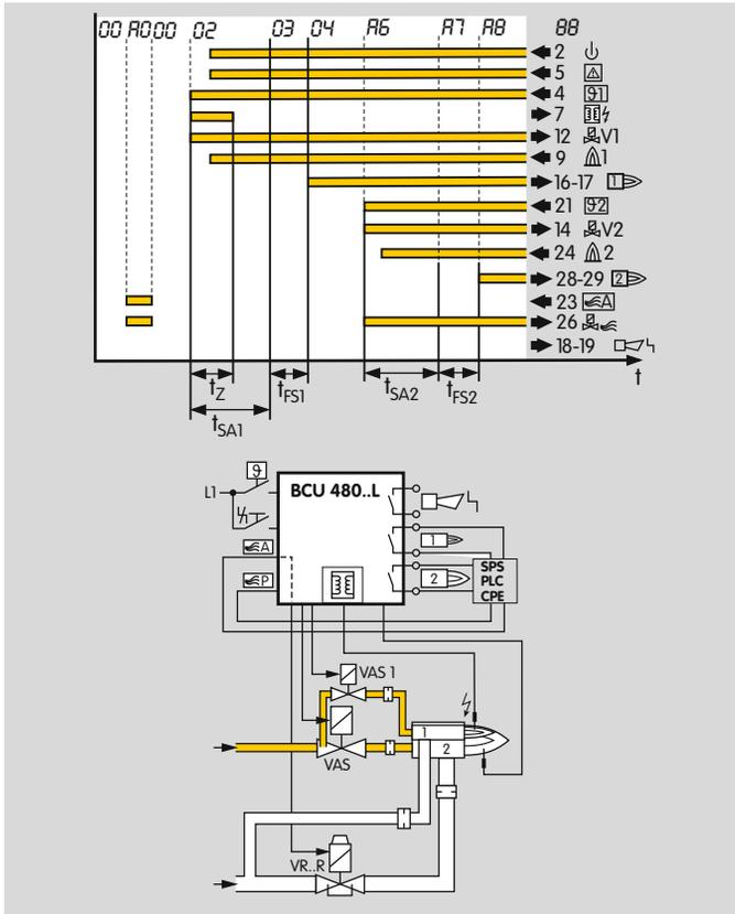
Parameter 30 = 2: The air valve opens simultaneously with valve V2.
