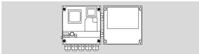
Open BCU and screw on with four screws ( $\varnothing$  4 mm, min. length 15 mm).
