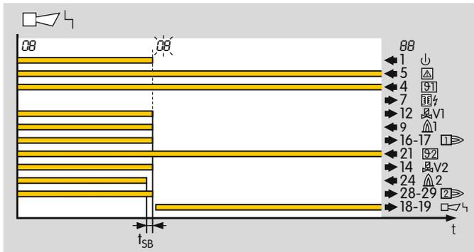
After a flame failure, the burner control unit performs a fault lock-out within the safety time during operation  $t_{SB}$ . This involves disconnecting the power from the gas valves and the ignition transformer. The fault signalling contact closes, the display blinks and shows the current program status, see table on page 27 (Program status and fault messages).
