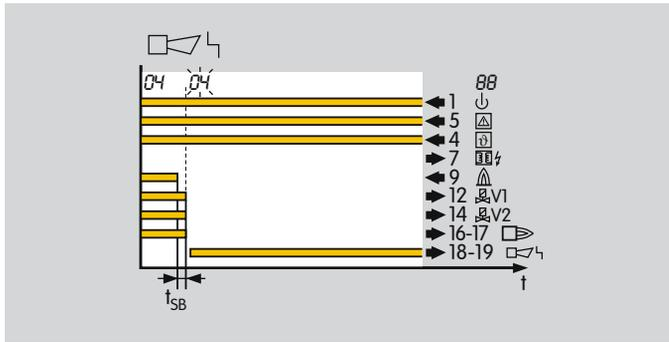
After an installation fault (flame failure or failure of air flow), the burner control unit performs a fault lock-out within the safety time during operation  $t_{SB}$ . This involves disconnecting the power from the gas valves and, if applicable, the ignition transformer. The fault signalling contact closes, the display blinks and shows the current program status, see table on page 39 (Program status and fault messages).
