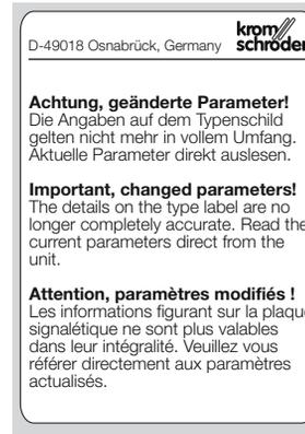
Affix on the connection diagram of the BCU following changes to unit parameters set at the factory.
