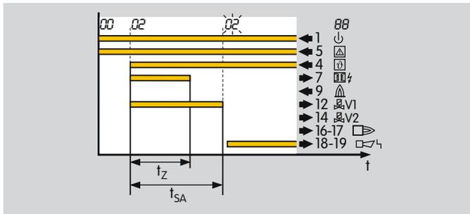
If no flame forms or, in the case of BCU 465, if the air flow fails during start-up, a fault lock-out is performed after expiry of time  $t_{SA}$ . The display blinks and shows the cause of the fault.
