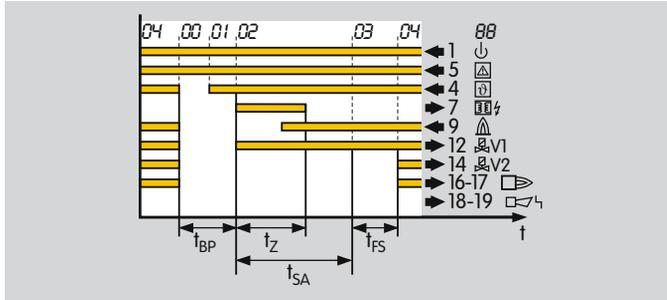
An immediate restart of the burner after a controlled shut-down is prevented by the pause time. The pause time starts when the burner is switched off. If a start-up signal ( $\vartheta$ ) is applied before expiry of this time, start-up is delayed until the end of the pause time.
