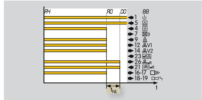
The air valve remains open for the programmed time after the start-up signal ( $\uparrow$ ) has been deactivated. The burner control unit closes the air valve after expiry of the post-ventilation time  $t_{NL}$ .
