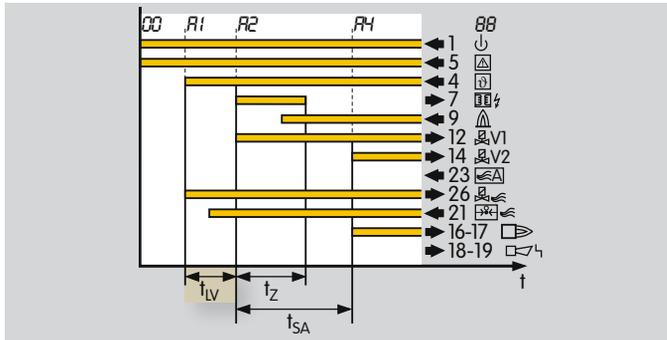
After the start-up signal ( $\vartheta$ ) has been applied and after the flame simulation check and “no flow” state check have been conducted successfully, the air valve is opened. Start-up of the burner commences as usual with no interruption of the air after expiry of the programmable pre-ventilation time  $t_{VL}$ .
