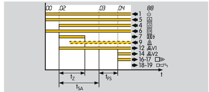
If the temperature in the furnace chamber drops below 750°C, the DI input must be disconnected from the electrical power supply and the furnace must then be operated with flame control.
