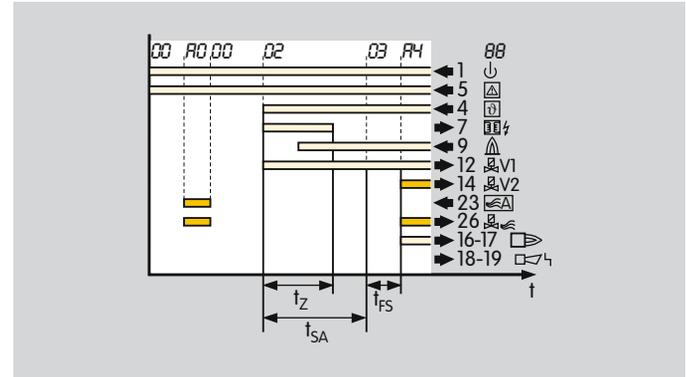
Parameter 30 = 2: The air valve opens simultaneously with valve V2.
