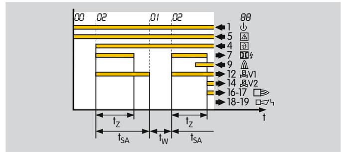
If several start-up attempts are set at the works and if the BCU detects an installation fault during start-up, it closes valve V1 after the safety time  $t_{SA}$  has expired and attempts to start up again. After the last programmed start-up attempt has been completed, the burner control unit conducts a fault lock-out. The display blinks and shows the cause of the fault.
