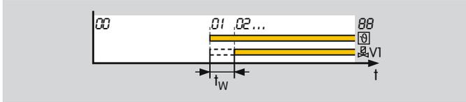
Once the start-up signal  $\vartheta$  has been applied, the waiting time  $t_W$  starts to elapse. During this time, a self-test is conducted to detect errors in internal and external circuit components. If no malfunction is detected, the burner will start up.
