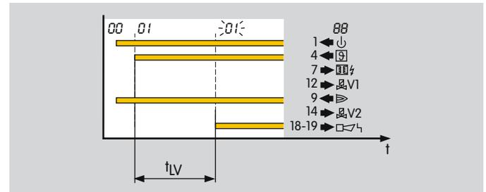
The flame simulation check of the burner is active until valve V1 is enabled.
