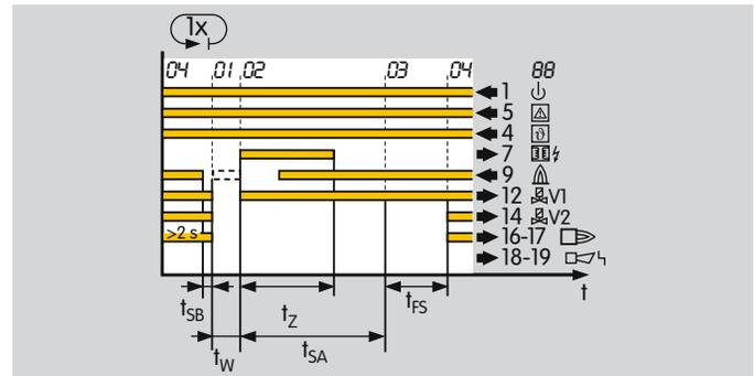
If the BCU detects an installation fault (flame failure or failure of air flow) after a minimum operating time of 2 s, the valves are closed and the operation signalling contact is opened within time  $t_{SB}$ .
