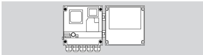
Open BCU and screw on with four screws (Ø 4 mm, min. length 15 mm).
