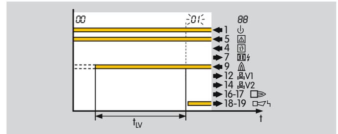
Flame simulation check on start-up (parameter 15 = 0):
