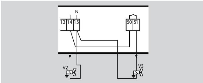
The following application describes a two-stage-controlled burner without a pneumatic air/gas ratio control system. V2 and the air valve are activated simultaneously. However, V2 may not be activated during purging.
