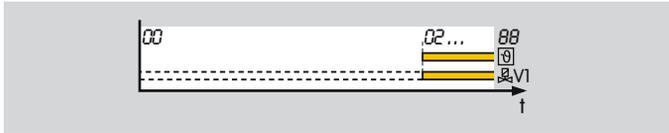
Parameter 15 = 1: The flame simulation check is conducted provided no start-up signal (0) is applied (during the so-called start-up position/standby). This allows fast start-up of the burner since there is no waiting time  $t_w$ .
