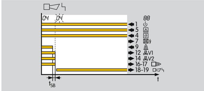
If the flame fails during operation, the valve outputs are disconnected within the safety time  $t_{SB}$ .
