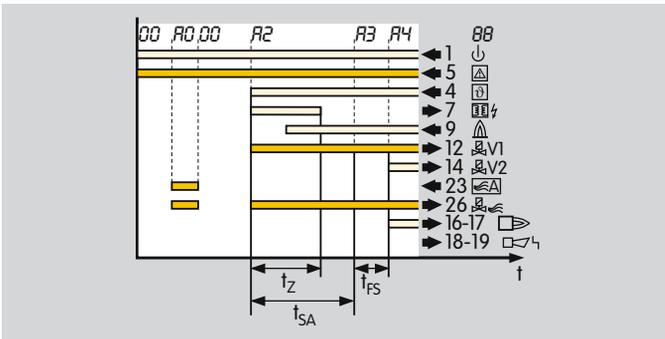
Parameter 30 = 1: The air valve opens simultaneously with valve V1.
