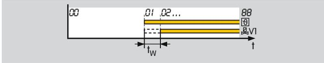
Parameter 15 = 0: The flame simulation check is conducted after applying the start-up signal (0) during the waiting time  $t_w$ .
