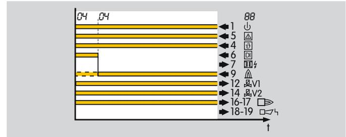
The burner remains in operation and the BCU performs flame control again (recommended in the case of ionization control or UV control with UVD).
