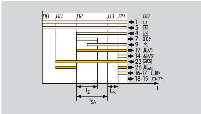
Parameter 30 = 0: The air valve opens if it is activated externally by input 23.
