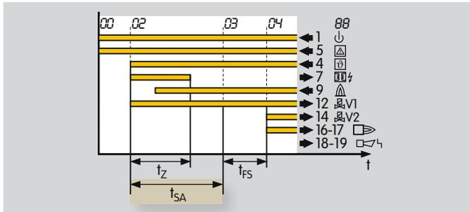
This indicates the safety time on start-up  $t_{SA}$  for the burner.
