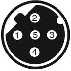
5-pin M12 built-in socket, D-coded
