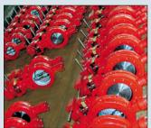
High performance butterfly valves are widely used in product and chemical tankers, offshore / on shore to NACE MR0175, oil and gas field chemical, petrochemical plants, and high pressure piping systems. The valves are complied with API 607 Edition 4 fire safety standards. Adoption of a spring-loaded soft PTFE seat gives flexibility and secures long life, even with frequent operation.
