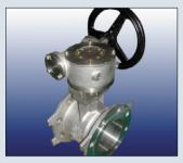
With a wide range of production, up to 4,000mm in size, the eccentric butterfly valves are developed for applications in waterworks, power plants, desalination plants and other similar industrial plants, with compliance to AWWA C-504, BS 5155 JIS B2064. They are available in a variety of body and disc materials. Rubber linings, epoxy coating and cathodic protection are available for installation in corrosive atmospheric conditions.
