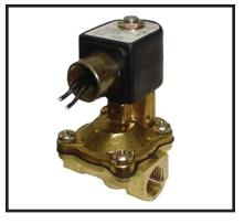
For best life and optimum performance, the Solenoid Valve should be mounted vertically upright, as illustrated in Figures 1 to 4, so as to minimize wear and reduce the possibility of accumulating foreign matter.
