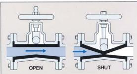
The rubber sleeve will be pressed to control the fluid when the clamp is operated with the manual handwheel.
