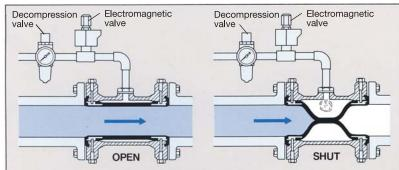
The rubber sleeve will be pressed to control the fluid when an operation air pressure 0.20 to 0.29 MPa higher than the pressure of the fluid is applied to the valve.
