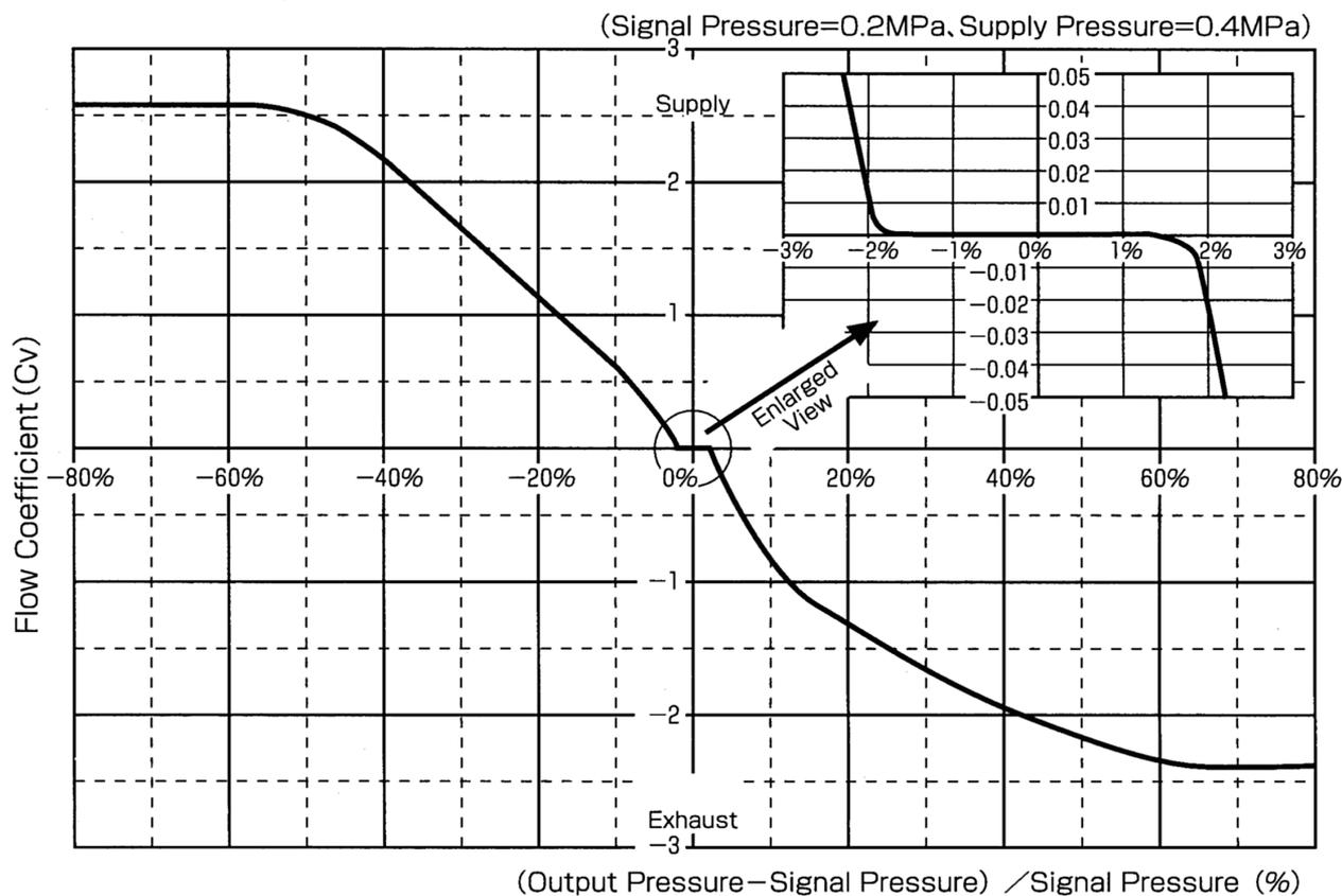
Figure 2 - Flow Characteristics
