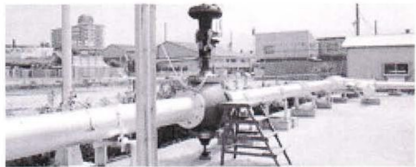
▲ Measurement device of valve flow capacity coefficient Cv (pneumatic type) MAX, Cv=10000
