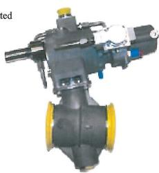
Meggitt's butterfly valves are designed for bleed air control on aero-derivative industrial gas turbine engines. This design was generated specifically for increased cycle life of the bearings and butterfly element while implementing precision control and position indication.
