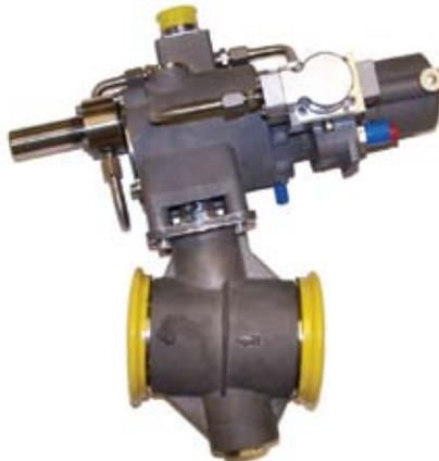
Meggitt's butterfly valves are designed for bleed air control on aero-derivative industrial gas turbine engines. This design was generated specifically for increased cycle life of the bearings and butterfly element while implementing precision control and position indication.
