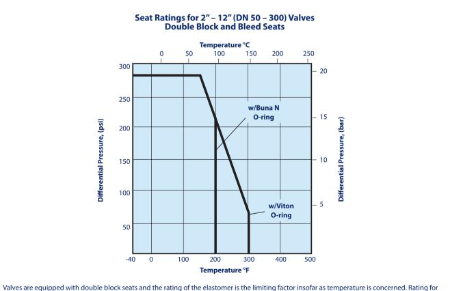
Valves are equipped with double block seats and the rating of the elastomer is the limiting factor insofar as temperature is concerned. Rating for standard elastomer Buna-N<sup>®</sup> material is -40°F to +200°F (-40°C to +93°C). Rating for Viton<sup>®</sup> elastomer is 0°F to 300°F (-17°C to +149°C). The standard DBB seat material is Filled PTFE.
