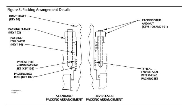
Refer to figure 3 which identifies the V280 packing components by key number (also see the Parts List section of this manual).
